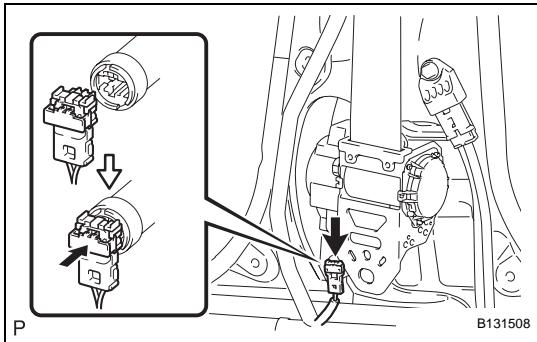
(b) Connect the pretensioner connector as shown in the illustration.
