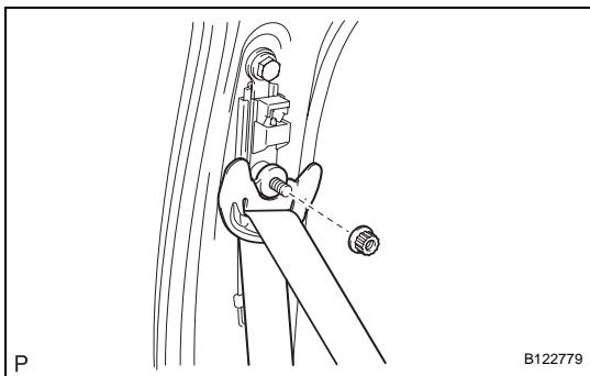
(c) Connect the outer belt with the shoulder anchor's bolt.
